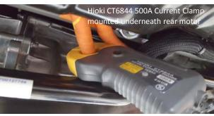
Pic of Hioki connection - DC/ DC to HV BUS
