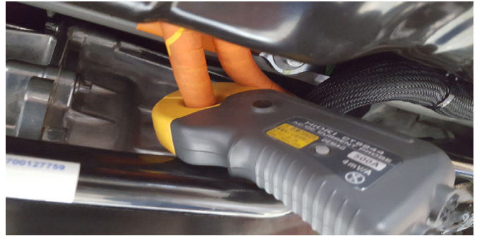
Pic of Hioki connection - High Voltage Ancillaries
