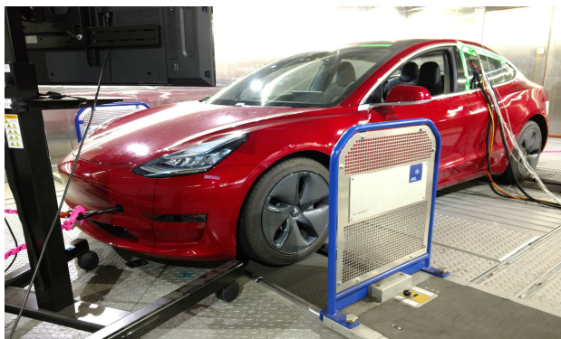
Pic of Hioki connection - Front Motor
