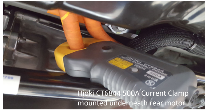
Pic of Hioki connection - High Voltage Ancillaries (Compressor)
