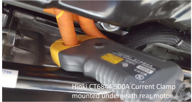
Pic of Hioki connection - High Voltage Ancillaries (Compressor)
