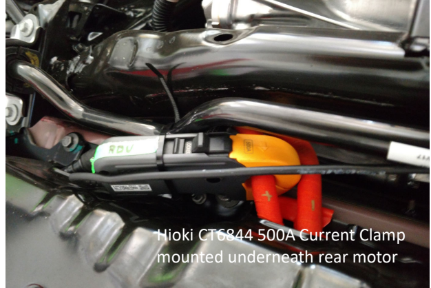
Pic of Hioki connection - High Voltage Ancillaries (Compressor)
