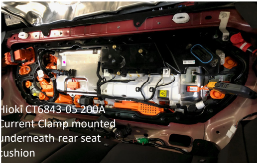
Pic of Hioki connection - DC/ DC to HV BUS
