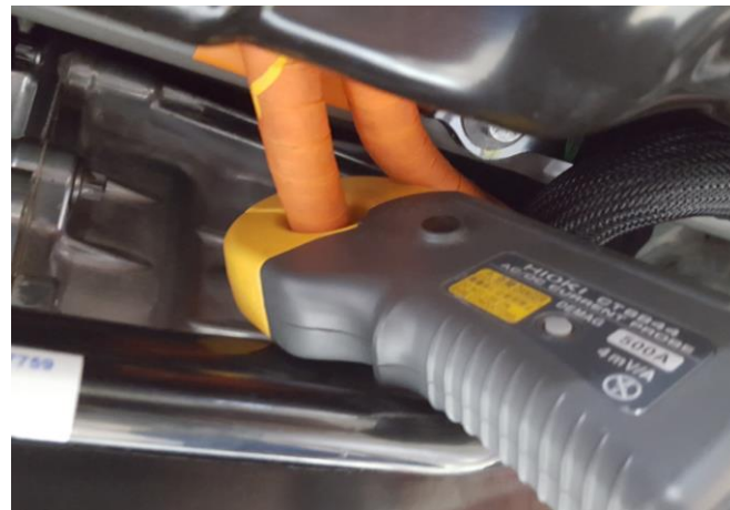
Pic of Hioki connection - Rear Motor
