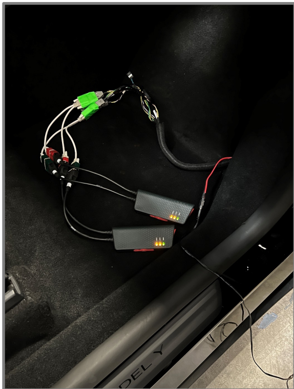
Dual Memorator connected via split cable
