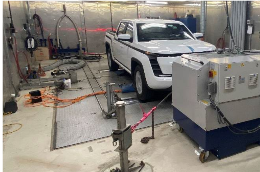
Figure 1. Endurance running on a dynamometer
