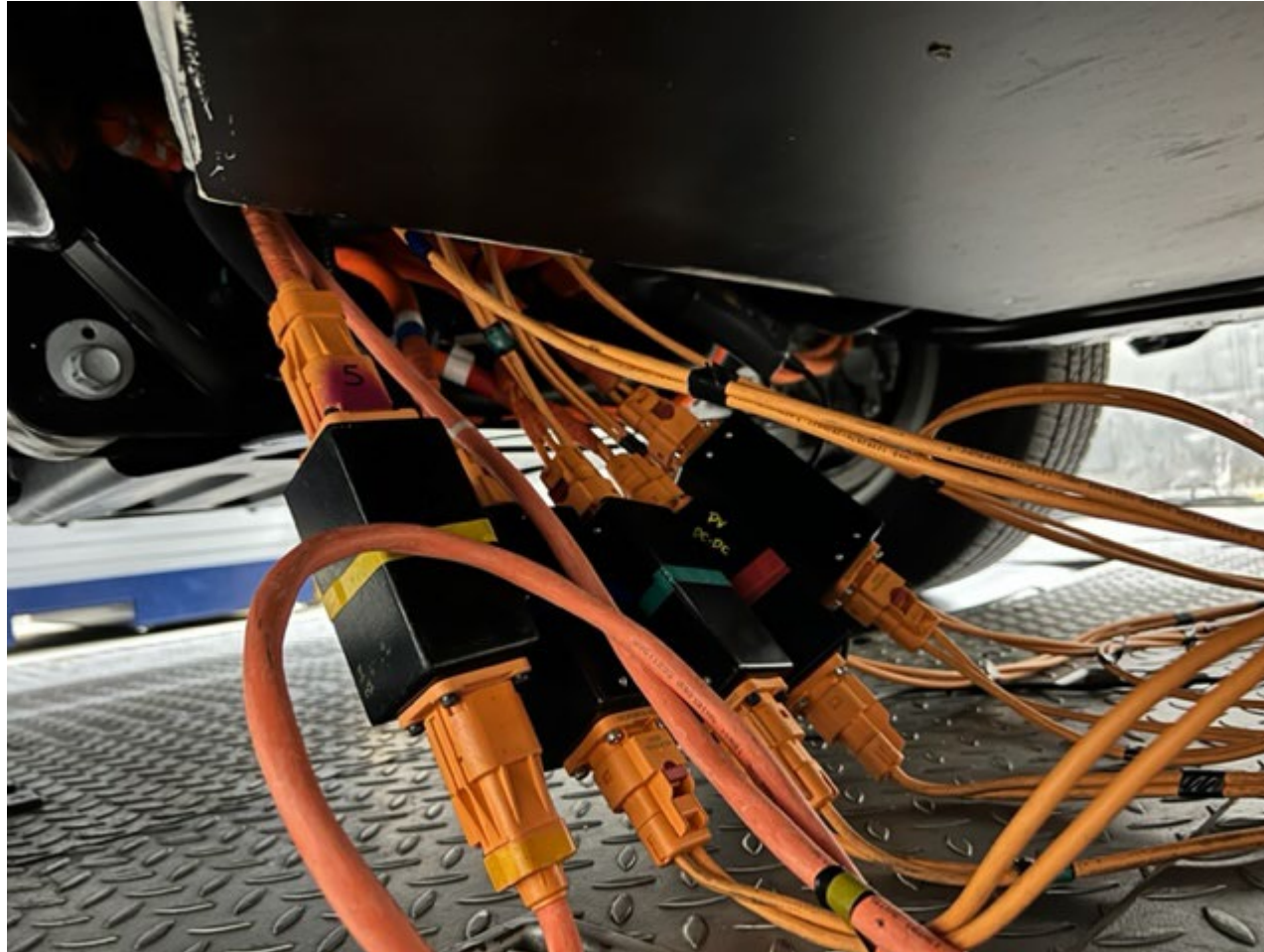
Figure 22. All break out box connectors connected to the vehicle
