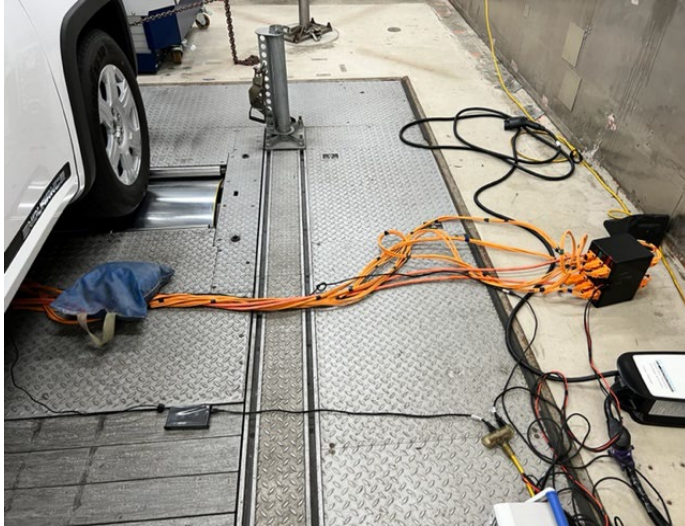
Figure 2. Breakout box and cables
