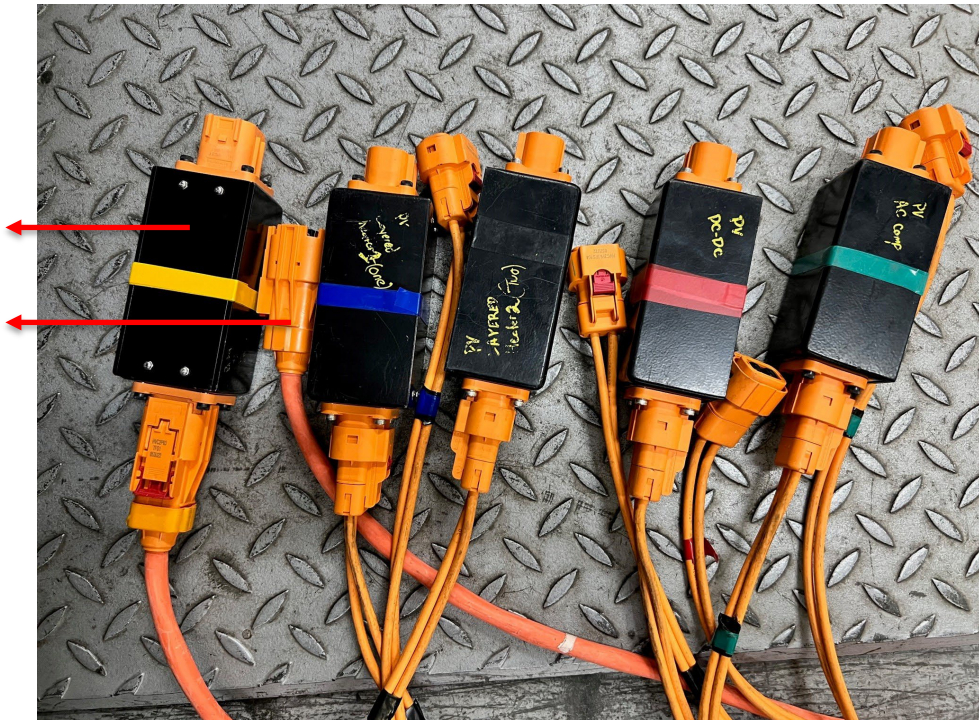
Figure 18. Male and female connectors from breakout box side
