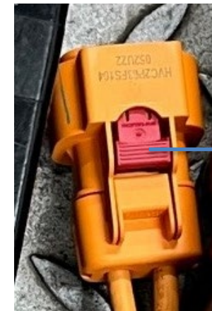
Figure 21. Female connector for DCDC, AC compressor, Cabin Heater, and Battery Heater
