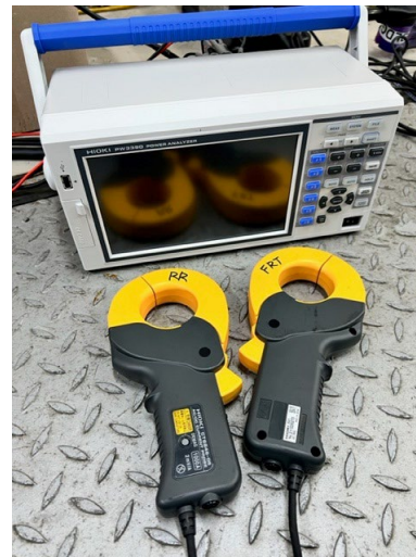
Figure 6. Power analyzer and current clamps
