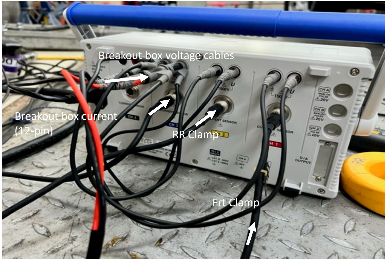
Figure 7. Power analyzer connection
