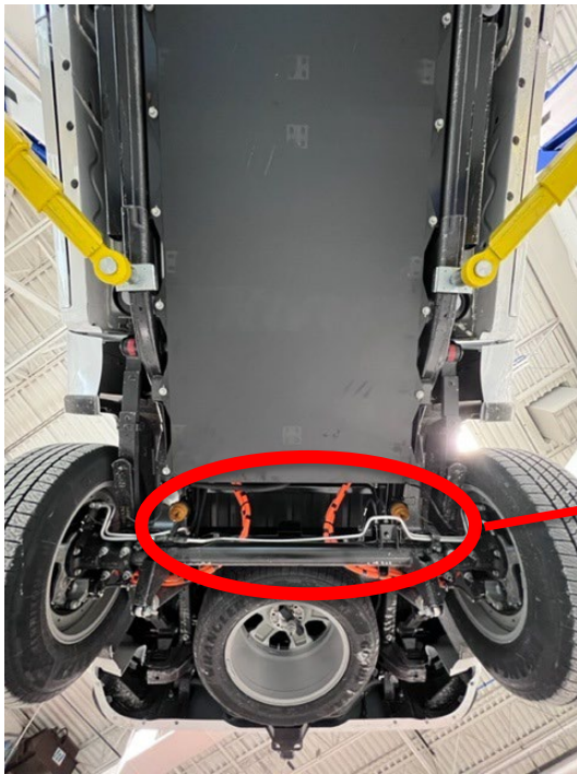
Figure 12. Location of the HV battery to rear inverter cables
